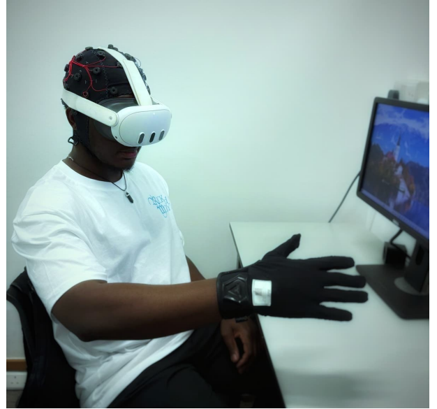
Figure 14: Experimental Setup with EEG headset, Quest 3 and bHaptics TactGloves
